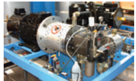
Maintenance-free sealing of dosing pumps for polyde and isocyanate in high-pressure reaction casting machines
