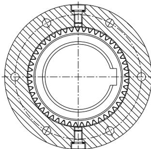
Illustration 29: Vertical position of locking screws
