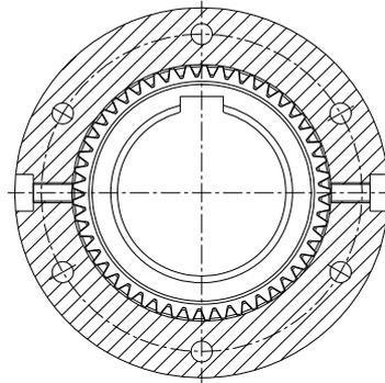
Illustration 28: Removing the locking screws and sealing washers
