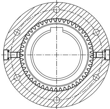
Illustration 27: Horizontal position of locking screws
