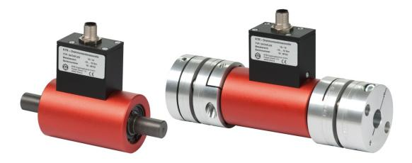
**DATAFLEX**<sup>®</sup> is a maintenance-free torque measuring shaft with integrated speed measurement. Combined with the steel lamina coupling **RADEX**<sup>®</sup>-**NC** the complete system forms a torsionally stiff, double-cardanic coupling with integrated measuring shaft.
