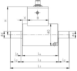
Illustration 1: DATAFLEX® torque measuring shaft
