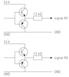
Illustration 16: output circuit of speed outputs
