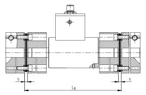
Illustration 7: assembly of the clamping hubs
