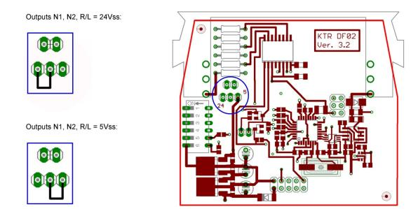
Illustration 17: modification of voltage level for the speed signal/direction signal
