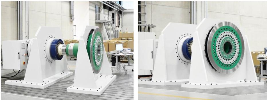
*Initial testing sample on the new test bench is a torque limiter having set a torque of more than 350,000 Nm*
